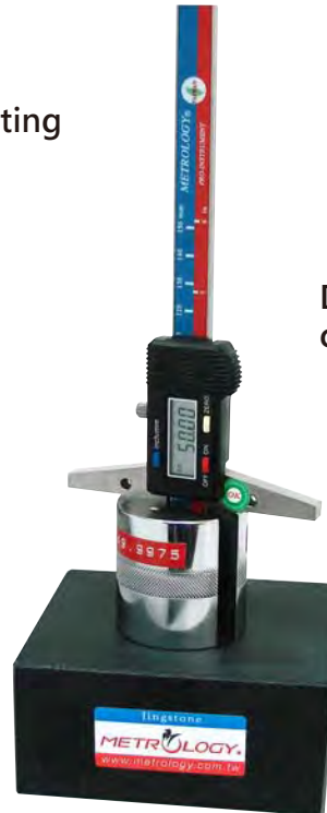
Depth caliper calibration
