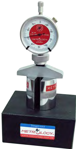
Dial Depth gauge calibration & zero setting
