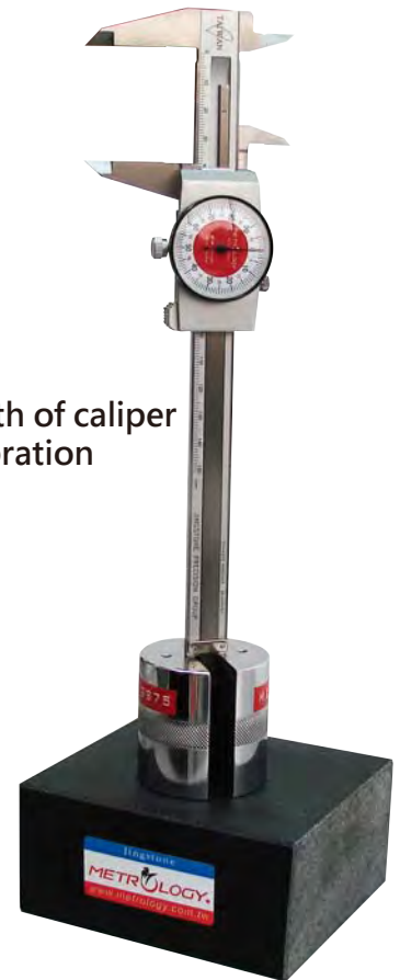
Depth caliper calibration
