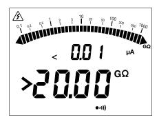
If, during an insulation measurement, the value to be measured exceeds the measurement range (which depends on the test voltage), the instrument so reports.
