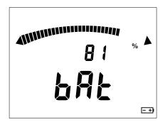
If the battery voltage is too low to ensure correct operation of the instrument, it so reports.
