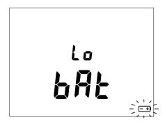
The batteries must then be replaced (see  $\S$  4.2)), since the battery life indication is no longer reliable.
