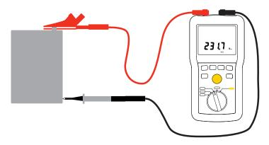
The instrument displays the voltage on the terminals. It detects whether the voltage is AC or DC and, if it is AC, displays its frequency.
