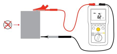
Use the leads to connect the device to be tested to the terminals of the instrument. The device to be tested must not be live.
