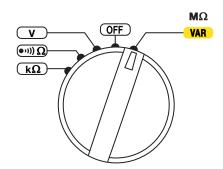
Set the switch to the  $M\Omega$  position.
