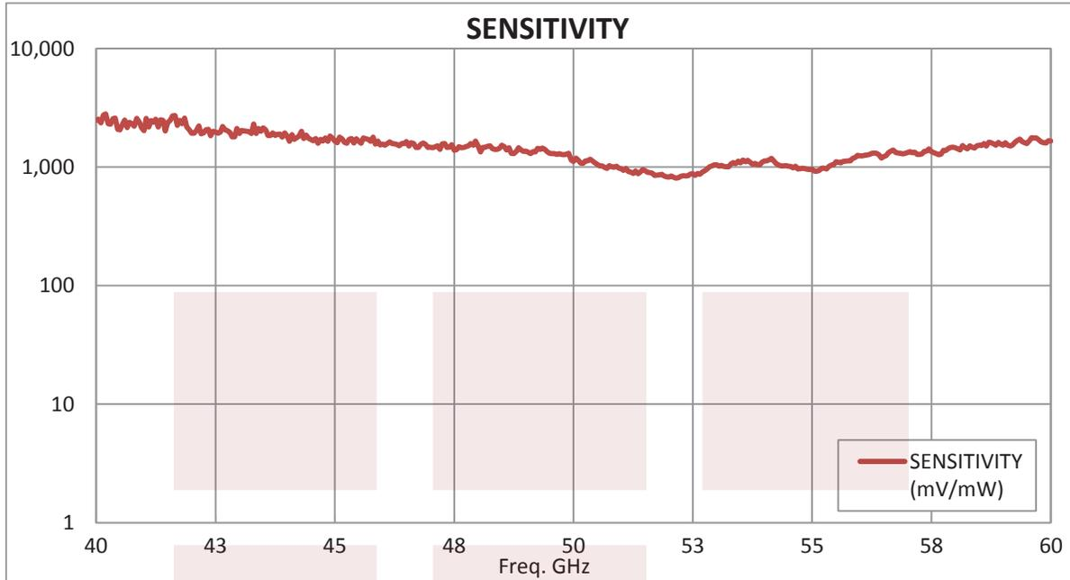
Zero Biased Waveguide Detector With WR-19 to SMA Female and Negative Video Out Operating From 40 GHz to 60 GHz U Band, UG-383/U from Fairview Microwave is in-stock and available to ship same-day. All of our RF/microwave products are available off-the-shelf from our ISO 9001:2008 certified facilities in Allen, Texas. Fairview Microwave is RF on-demand.
