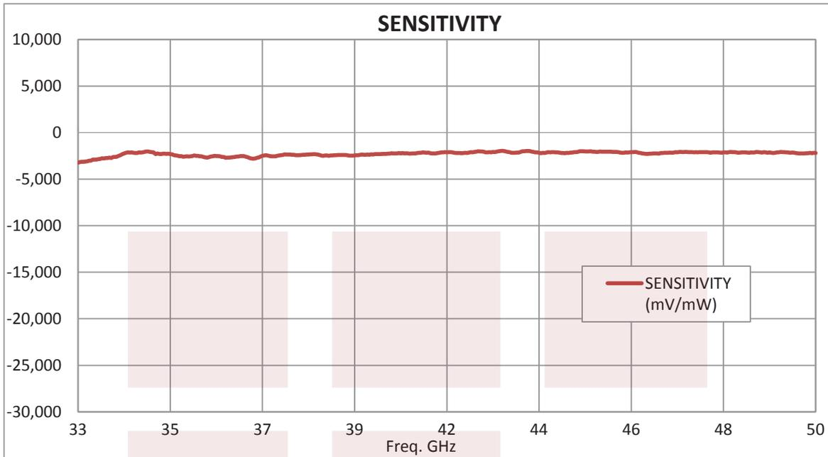
Zero Biased Waveguide Detector With WR-22 to SMA Female and Negative Video Out Operating From 33 GHz to 50 GHz Q Band, UG-383/U from Fairview Microwave is in-stock and available to ship same-day. All of our RF/microwave products are available off-the-shelf from our ISO 9001:2008 certified facilities in Allen, Texas. Fairview Microwave is RF on-demand.
