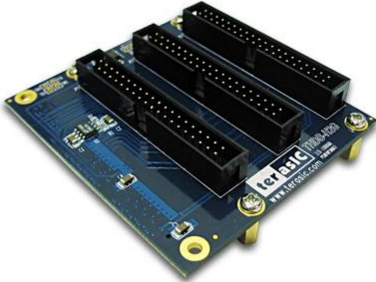
The THDB-H2G (HSMC to GPIO Daughter Board) board is designed to fan out the High Speed Mezzanine connector (HSMC) I/Os to three 40-pin expansion prototype connectors, which are compatible with Altera DE2/DE1/DE0 expansion headers. Users can connect up to three Altera DE2/DE1/DE0 boards (or associated daughter cards) onto a HSMC-interfaced host board via the THDB-H2G board.
