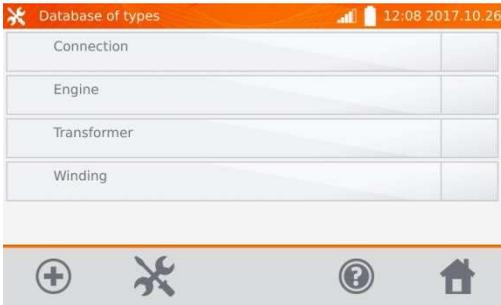
The meter has 4 default types saved in its memory. Use **+** button to add a new type of the tested object.
