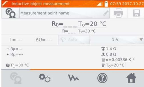
8 Connect the meter to the tested object. Press **START/STOP**.
