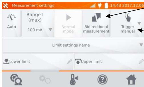
Switching Unidirectional/Bidirectional measurement.
