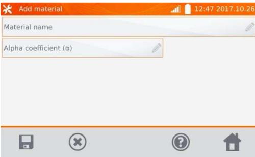
Enter and save the material and  $\alpha$  coefficient, using the same method as described in section 2.2.4.
