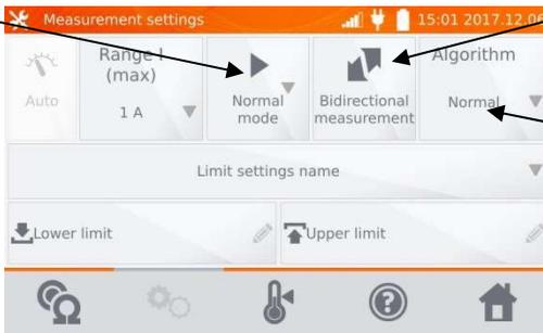
Switching Unidirectional/Bidirectional measurement.
