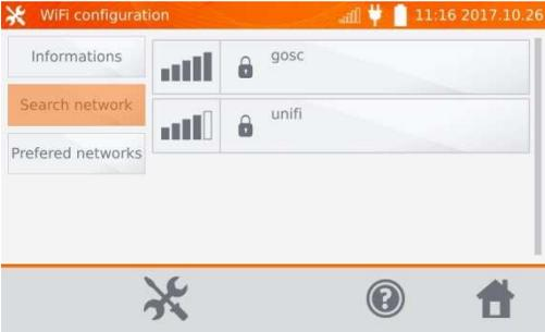
The meter detected networks secured by password. Click the name of the network to enter the password.
