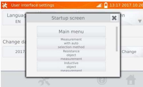
Click the selected startup screen (the screen will be automatically shown after turning on the meter). This feature is useful for making measurements of a given type for a longer period.
