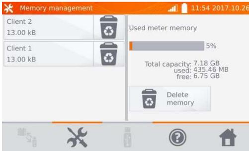
This option allows you to read the % of the used memory and to clear it: after clicking **Delete memory** all clients are deleted with their objects and measurement results. By pressing button
