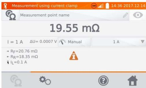
In addition to the resistance, the meter also displays the value of current measured with clamps.
