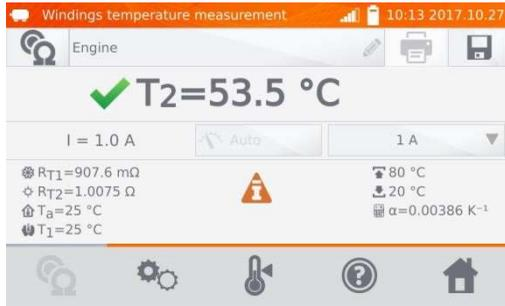
$R_{T1}$  – resistance of the cold winding
