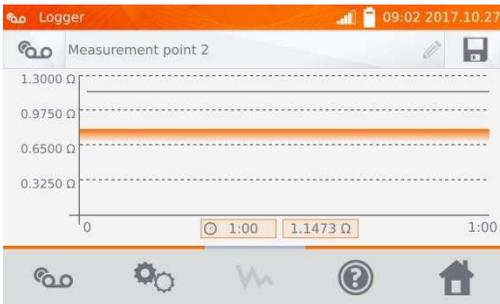
Use button to display the graph of resistance over time - both during the logging process and after its completion.
