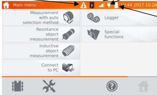
Battery charge level, x – indicates empty battery or no battery in the compartment.
