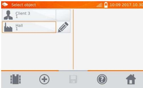
After adding and saving the object (also subobjects if necessary), click **+** button to add the measurement point.
