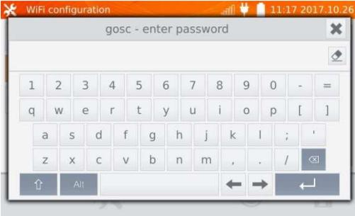
Enter the password and confirm it by pressing
