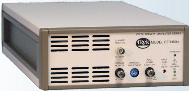
The Trek Model PZD350A is a high-voltage DC-stable piezo driver/amplifier designed to provide precise control of output voltages in bipolar or unipolar ranges that are customer specified within a range of available settings. It is configured as a noninverting amplifier with a variable DC gain. An inverting amplifier configuration is also available.
